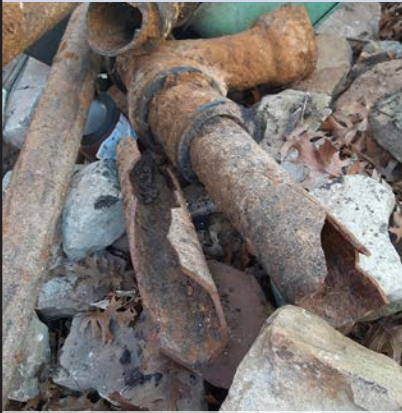
Corroded sewer pipes
